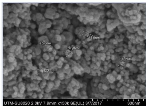
Figure 12: FESEM micrograph for couple catalyst \text{TiO}_2/\text{ZrO}_2 (90:10) calcined at 700^\circ\text{C}
