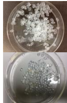
(a) Alginate beads crosslinked with CNW and (b) alginate beads without CNW
