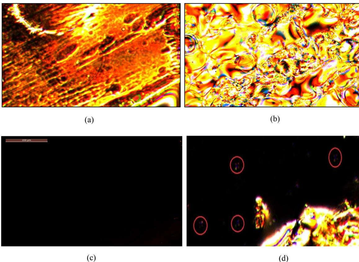
**Figure 3** 5CB showing thermal scenario during heating and cooling process: (a) nematic phase at 25.0°C (b) nematic-isotropic phase at 35.0°C (heating) (c) dark region of isotropic phase (d) isotropic-nematic phase at 35.0°C (cooling)
