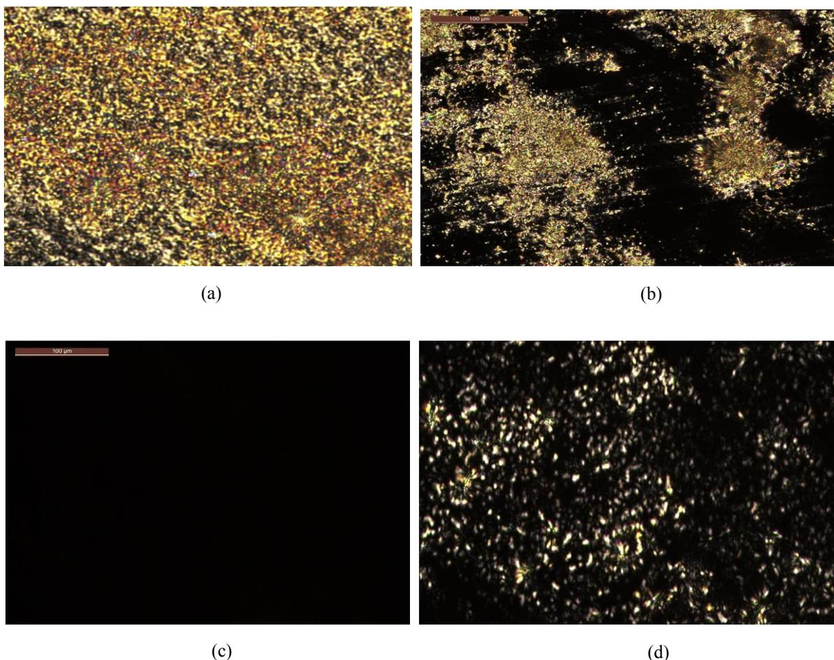
**Figure 4** 5 w/v% of SiO<sub>2</sub>/5CB showing thermal scenario during heating and cooling process: (a) nematic phase at 25.0°C (b) nematic-isotropic phase at 35.0°C (heating) (c) dark region of isotropic phase (d) isotropic-nematic phase at 35.0°C (cooling)
