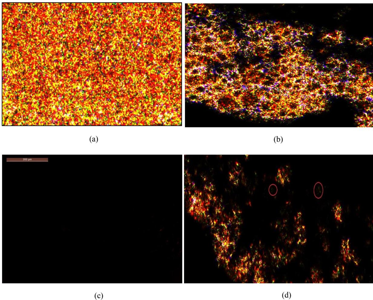
**Figure 5** 10 w/v% of  $\text{SiO}_2/5\text{CB}$  showing thermal scenario during heating and cooling process: (a) nematic phase at  $25.0^\circ\text{C}$  (b) nematic-isotropic phase at  $35.0^\circ\text{C}$  (heating) (c) dark region of isotropic phase (d) isotropic-nematic phase at  $35.0^\circ\text{C}$  (cooling)
