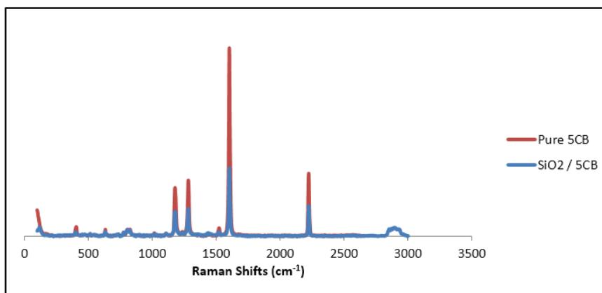
**Figure 6** Raman shifts for pure 5CB and 10 w/v%  $\text{SiO}_2/5\text{CB}$
