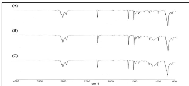
**Figure 2** ATR-IR spectra of (A) pure 5CB (B) 5 w/v% SiO<sub>2</sub>/5CB (C) 10 w/v% SiO<sub>2</sub>/5CB
