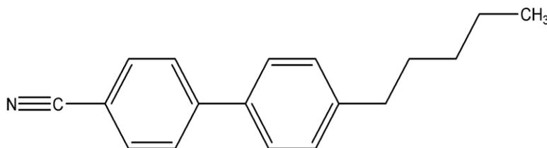
Figure 1.1 Chemical structure of 5CB
