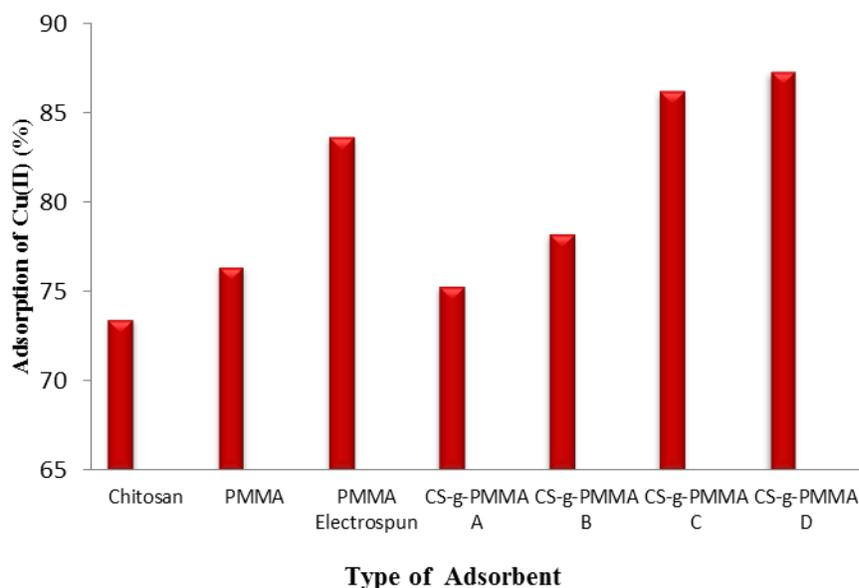
**Figure 10** Percentage of adsorption of Cu(II) using various adsorbents
