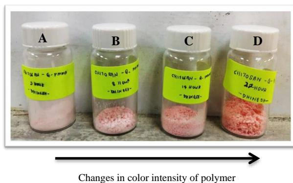
**Figure 4** The product obtained from grafting of PMMA on chitosan at 2 hour (A), 8 hour (B), 14 hour (C) and 22 hour (D).
