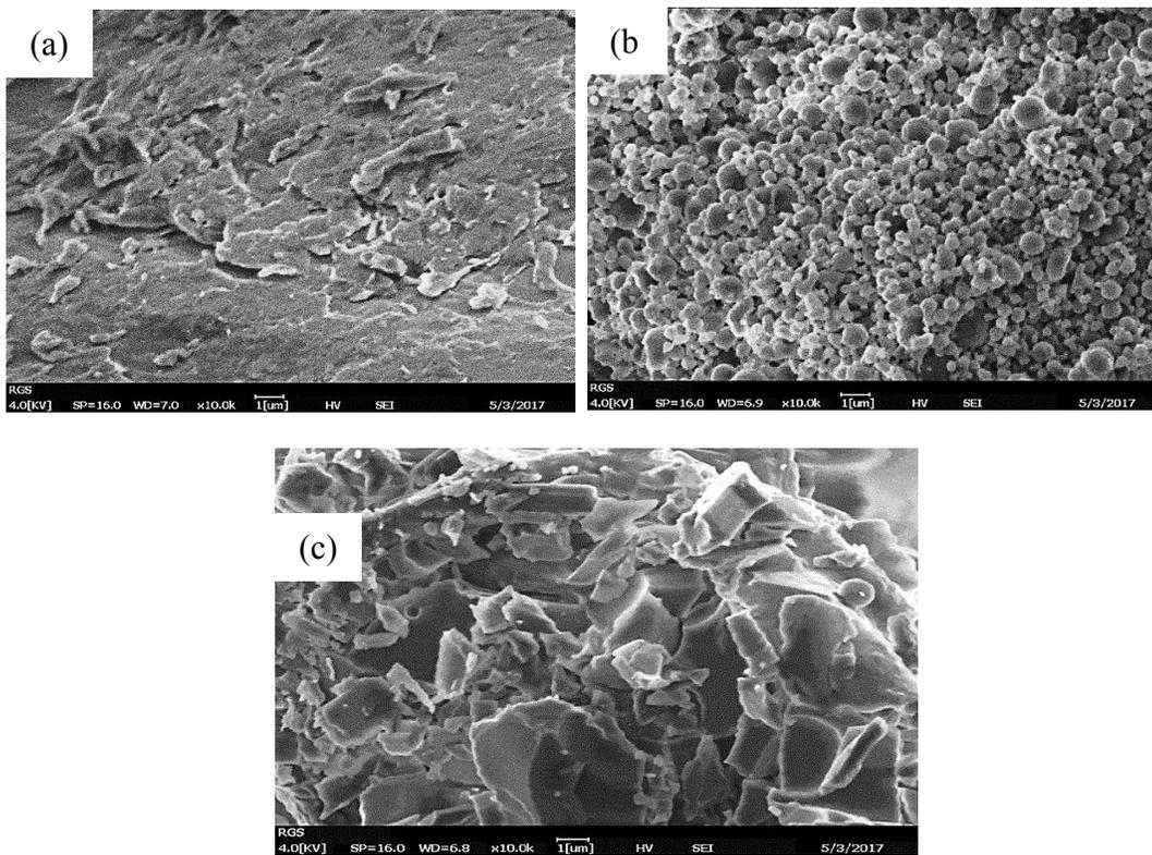
**Figure 7** SEM micrographs of (a) CS (x 10), (b) PMMA (x 10) and (c) CS-g-PMMA (x 10).
