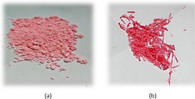
**Figure 8** Comparison on physical property of PMMA in (a) powdered-form and (b) electrospun-form obtained via electrospinning technique.
