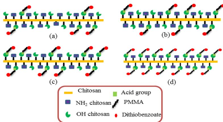
**Figure 5** The quantities of PMMA homopolymers grafted on chitosan at (a) A, (b) B, (c) C and (d) D.
