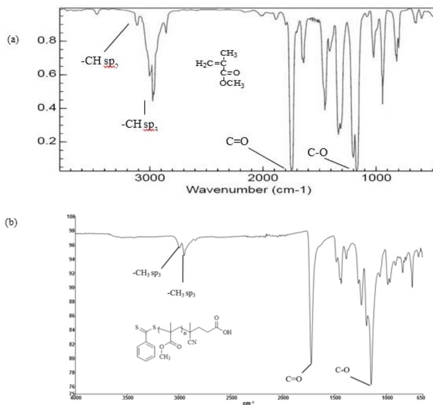
**Figure 1** IR spectrum of (a) MMA and (b) PMMA
