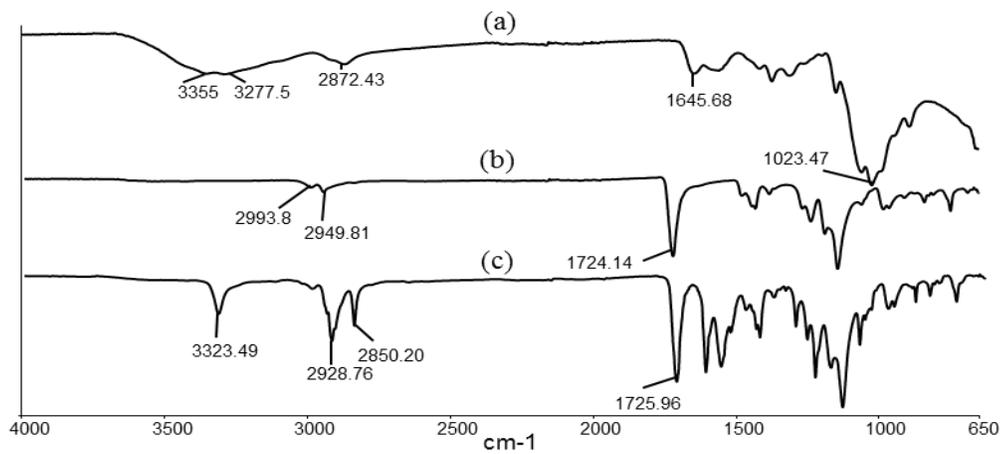
Figure 3 The ATR spectrum of (a) chitosan, (b) PMMA macro RAFT agent and (c) CS-g-PMMA.
