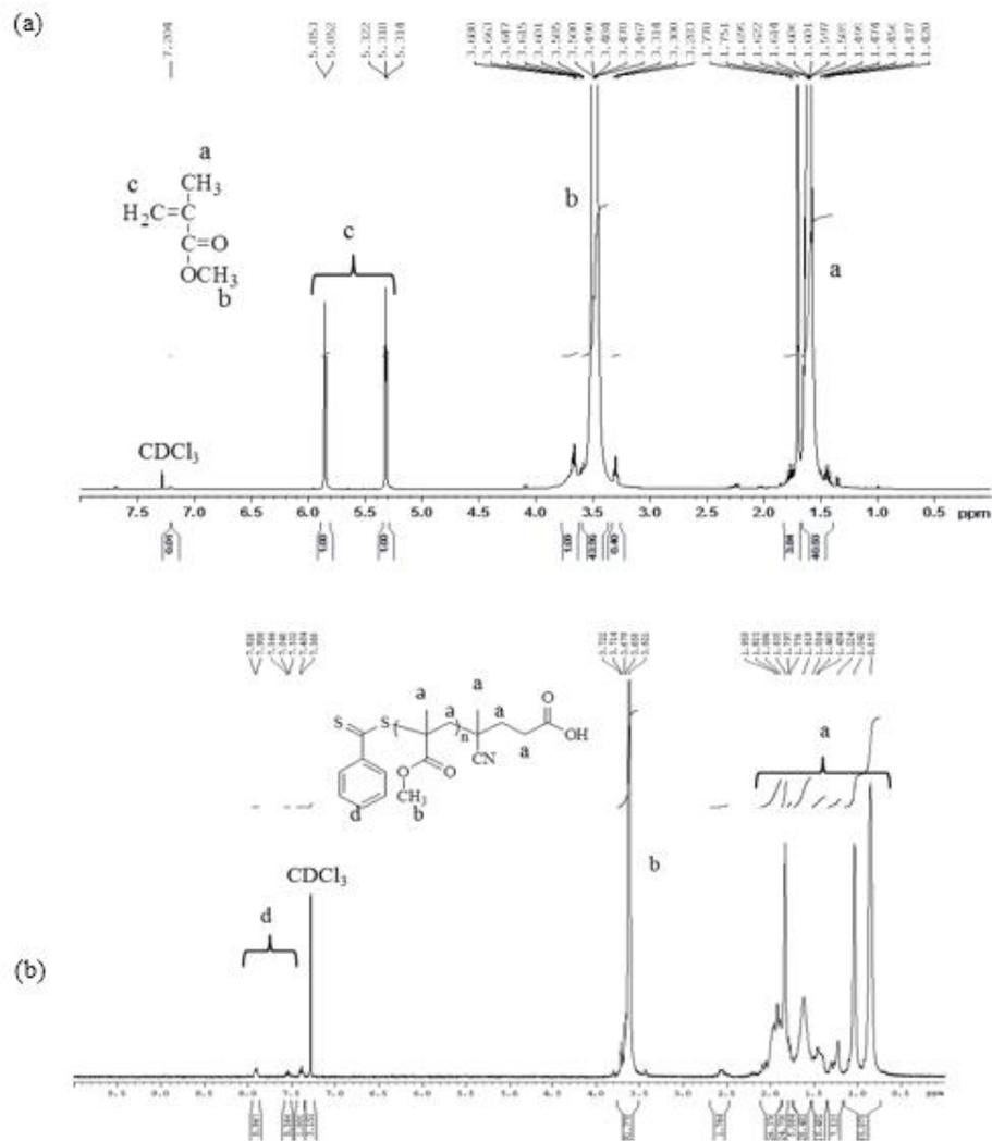
Figure 2 <sup>1</sup>H-NMR spectrum of (a) MMA and (b) pure PMMA
