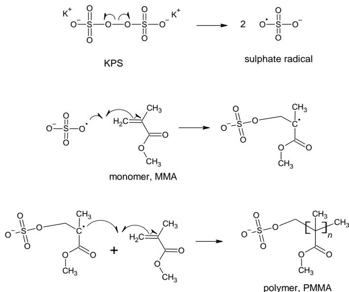
**Figure 2** Proposed mechanism of PMMA.
