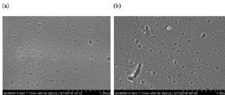
**Figure 10** Morphology image for clear surface of PMMA-spiropyran- lemongrass oil using FESEM at (a) and (b) 50k magnification.
