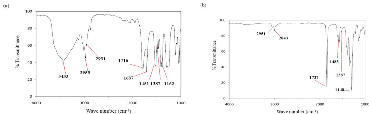
**Figure 3** FTIR spectra for (a) MMA and ATR spectrum for (b) PMMA.
