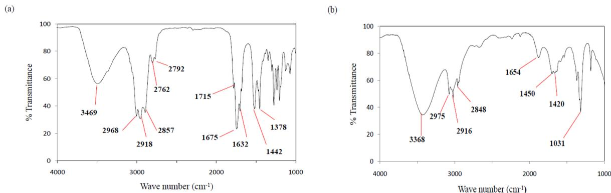
**Figure 1** FTIR spectra of lemongrass oil extracted using (a) steam distillation and (b) solvent extraction.
