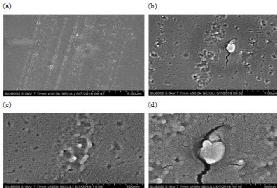
**Figure 9** Morphology image for rough surface PMMA-spiropyran- lemongrass oil using FESEM at (a) 10K magnification, (b) 50K magnification, (c) 100K magnification, (d) 150K magnification.
