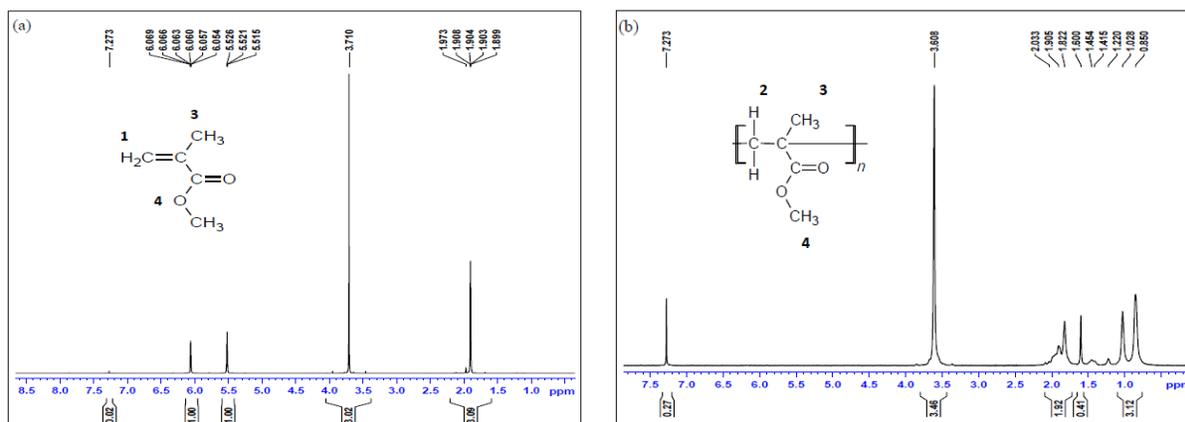
**Figure 4**  $^1\text{H-NMR}$  spectra for (a) MMA and (b) PMMA in  $\text{CDCl}_3$ .
