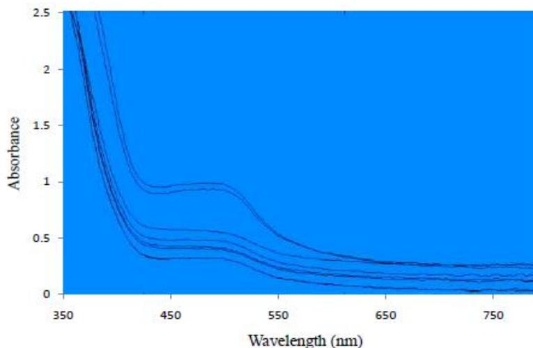
**Figure 8** UV-Vis spectra spectrum of PMMA embedded with spiropyran and lemongrass oil.
