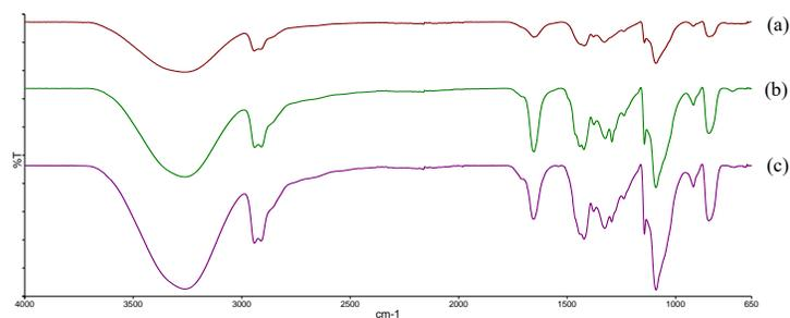
**Figure 3** FTIR spectra of (a) PVA; (b) PVA/PVP; (c) PVA/PVP-violacein by using casting method.
