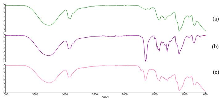
**Figure 4** FTIR spectra of (a) PVA; (b) PVA/PVP; and (c) PVA/PVP-violacein membrane by using electrospinning method.
