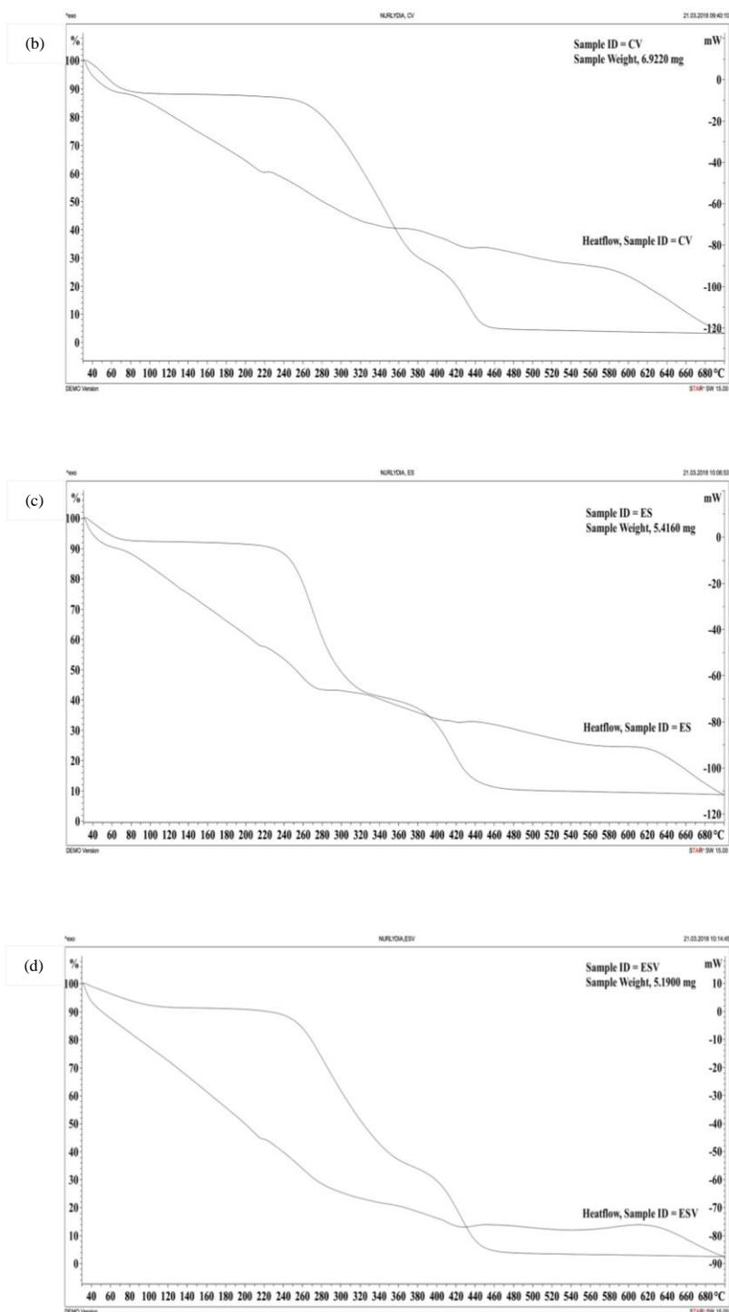
**Figure 6** TGA-DSC plot of (a) casted PVA/PVP; (b) casted PVA/PVP-violacein; (c) electrospun PVA/PVP; and (d) electrospun PVA/PVP-violacein membranes.
