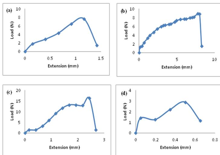
**Figure 2** (a) The tensile strength of (a) cast PVA/PVP membrane; (b) cast PVA/PVP-violacein membrane; (c) electrospun PVA/PVP membrane; and (d) electrospun PVA/PVP-violacein membrane.
