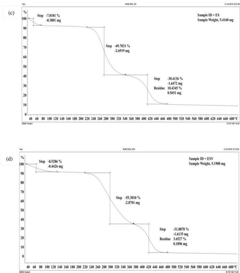
**Figure 5** TGA plot of (a) casted PVA/PVP; (b) casted PVA/PVP-violacein; (c) electrospun PVA/PVP; and (d) electrospun PVA/PVP-violacein membranes.
