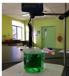
Process of plating copper substrate in KFJ-20 (EN)
