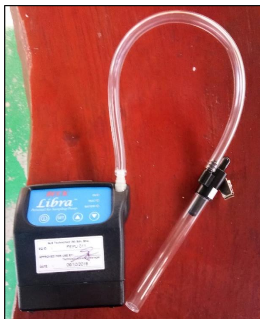
Figure 3. Portable air sampler pump (Bulk Libra pump L-4) used for active sampling
