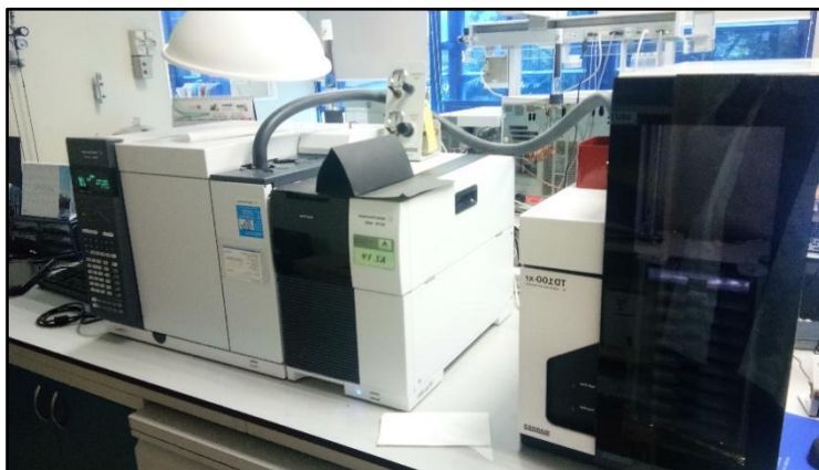
Figure 4. TD-GC-MS instrument that was used for analysis of VOCs
