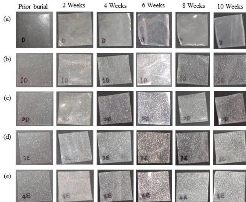
Fig. 5 Biodegradable images of the films prior and after soil burial test; (a) pure PLA, (b) PLA/C1, (c) PLA/C2, (d) PLA/C3 and (e) PLA/C4.
