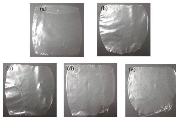
Fig. 7 Visual comparison of the transparency of (a) pure PLA, (b) PLA/C1, (c) PLA/C2, (d) PLA/C3 and (e) PLA/C4
