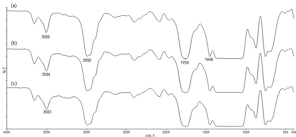
Fig. 1 FTIR spectra of (a) pure PLA, (b) PLA/C1 and (c) PLA/C2
