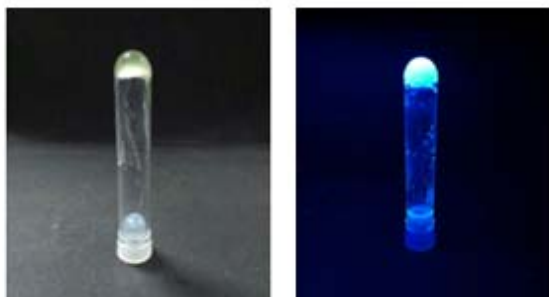
Figure 4 (a) Inverted test flow of \text{BTA}_{1+2} organogel and (b) \text{BTA}_{1+2} organogel observed under hand-held UV lamp 365 nm
