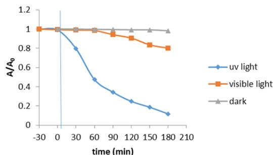
Figure 7 Comparison of MB photodecolourization in the dark, visible and UV light irradiation by ZnO-NPs
