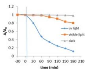
Comparison of MB photodecolourization in the dark, visible and UV light irradiation by ZnO-NPs
