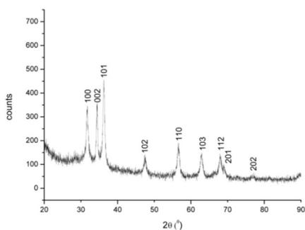
Figure 3 XRD pattern of hexagonal wurzite ZnO-NPs
