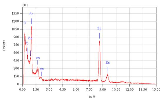
Figure 6 EDX spectrum for ZnO-NPs
