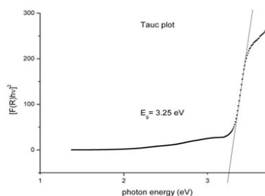
Figure 2 Plot of  $(F(R)hv)^2$  vs  $hv$
