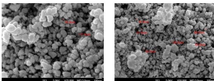
Figure 5 FESEM micrograph of ZnO-NPs (a) higher magnification (b) lower magnification
