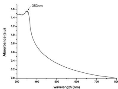
Figure 1 UV-Vis spectrum of ZnO-NPs
