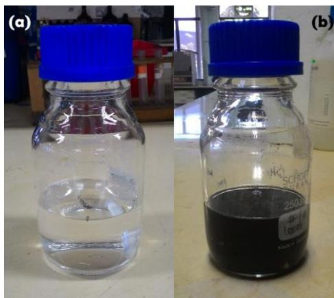
**Figure 2** Color of dope polymer solution (a) dope PSEBS solution (b) dope PSEBS-GO solution
