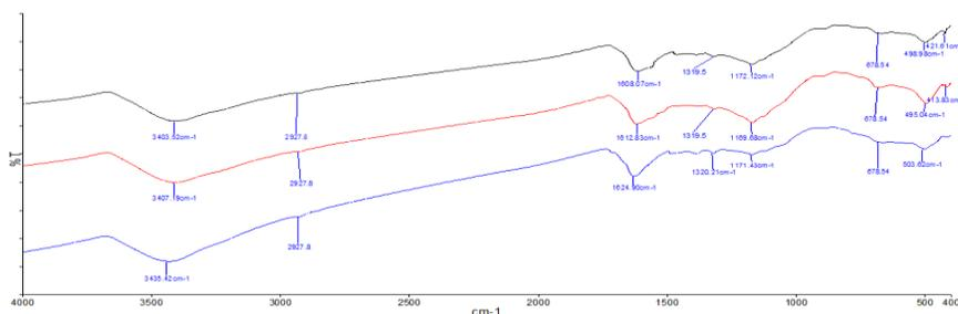
Figure 3 FTIR spectra of ZHLAC45, 55 and 65
