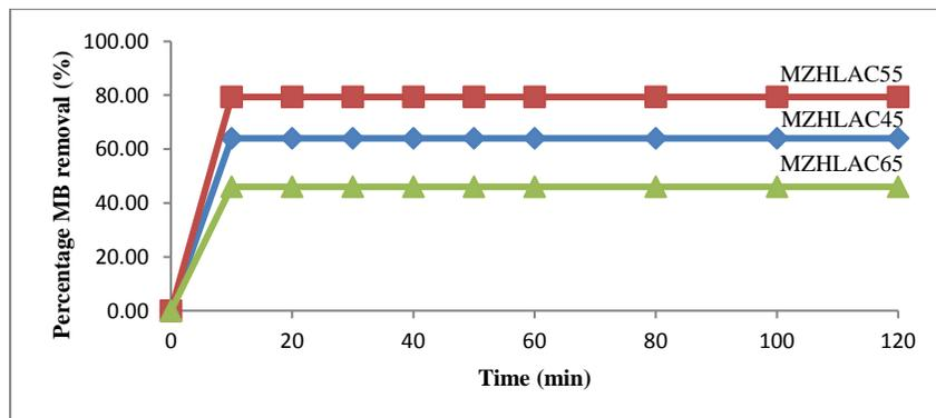
Figure 11 Effect of adsorption capacity of MB onto MZHLAC45, 55, and 65
